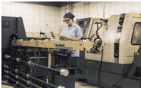
CNC Lathes produce accurately turned microwave parts
